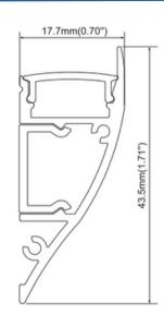
Experience dynamic lighting with Zortech LED's AL62 wall up lighting aluminum extrusion. Seamlessly blend LED strips at right angles for an easy and attractive way to add up lighting on any wall. This design conceals the LED strip, so you'll see just the light and not diodes.
