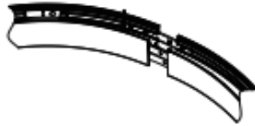
Step 02: Connecting the curved profile by connector
