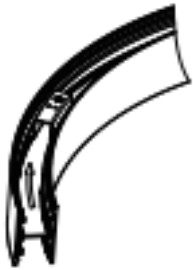
Step 01: Slide the U shape hanging clip into the profile
