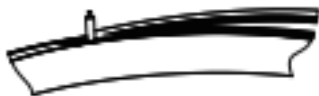
Step 07: Press the curved cover(after drilling the hole) into the profile(up light)
