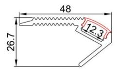
Step into sophisticated lighting with Zortech LED's AL22 stair nosing aluminum extrusion. Seamlessly incorporate LED strips for a sleek and practical lighting solution that adds safety and style to staircases.
