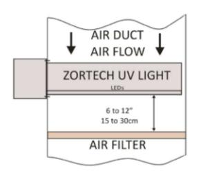
UV595 and 395 reduces biological contaminants such as bacteria, mold and allergens in indoor air using UVC light. The system is installed in the duct work of the central air system.
