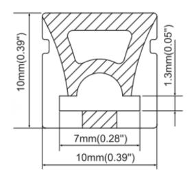
Experience dynamic lighting with Zortech LED's S1010-T small silicone extrusion. Seamlessly blend LED strips for a versatile and captivating "do it yourself" neon type lighting, great for indoor and outdoor applications.
